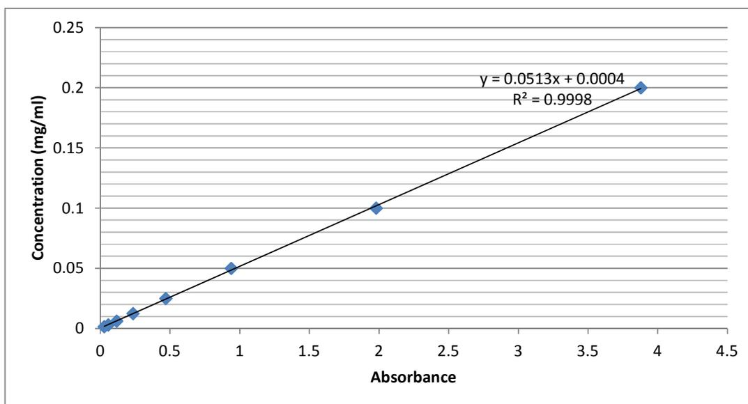
Fig. 2. Calibration curve of pure metronidazole in 0.1N HCL at 277 nm
