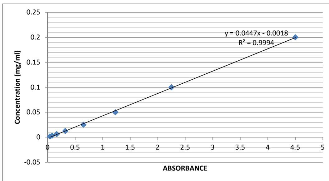
Fig. 3. Calibration curve of pure metronidazole in 6.8 simulated intestinal fluid at 322 nm
